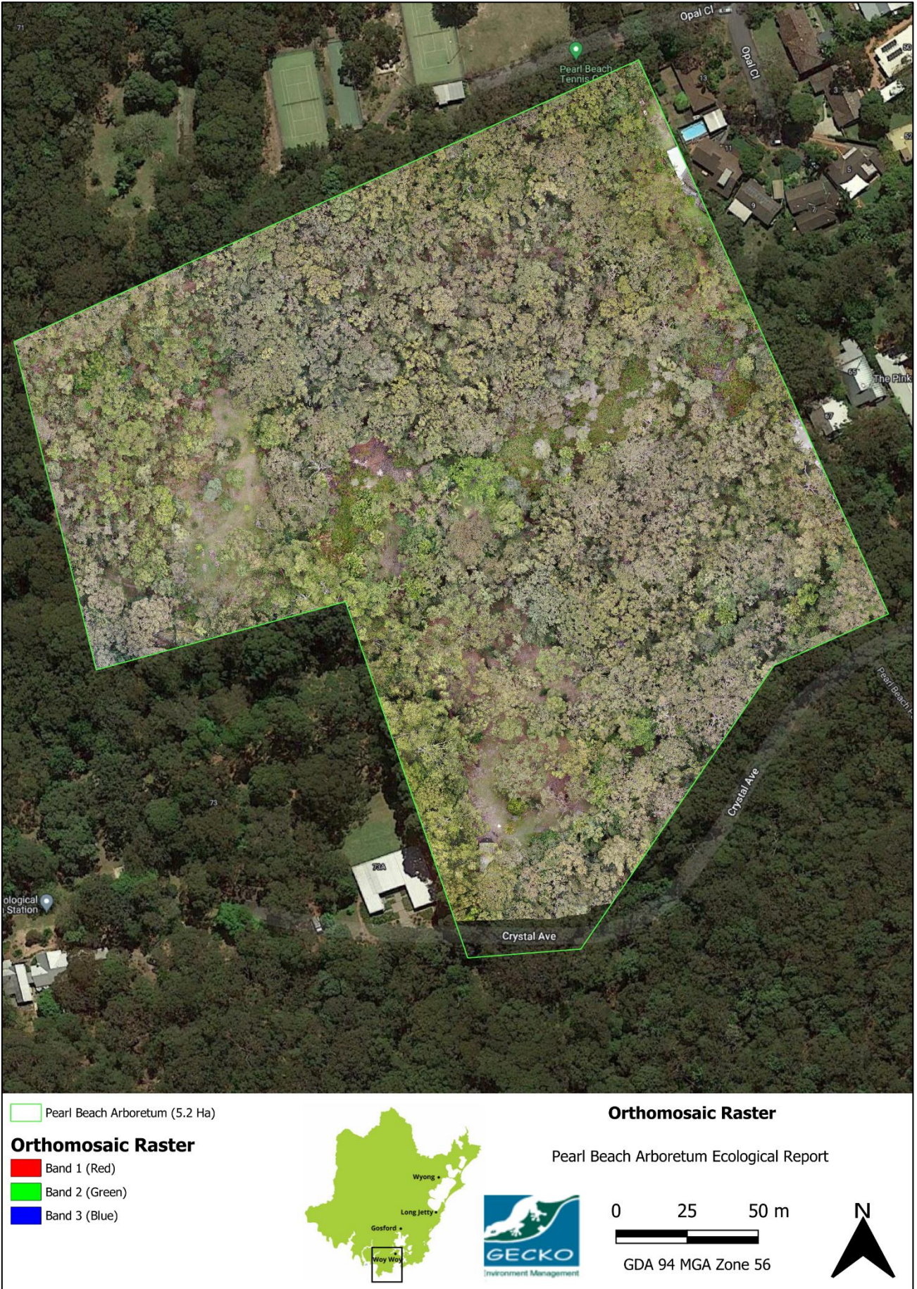
Figure 5: UAV acquired imagery processed into a high resolution orthomosaic GEOTIFF raster of the study area.
