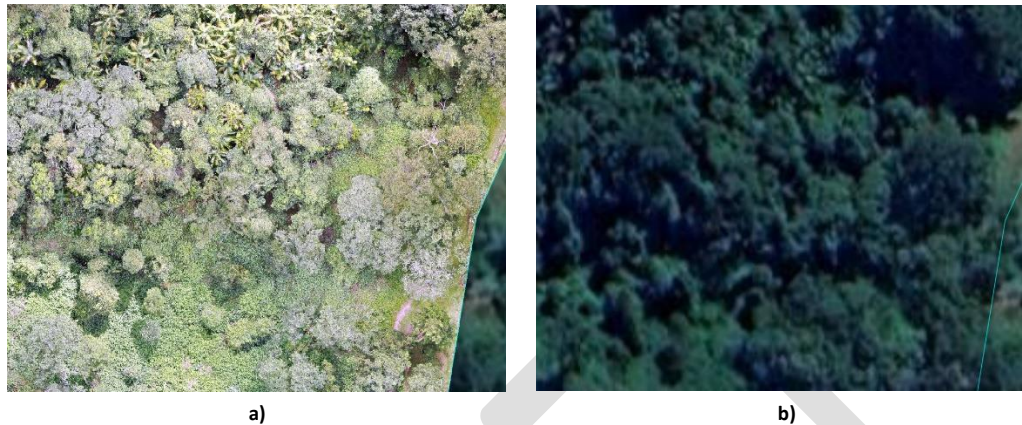
Figure 3: Same portion of a study area at different spatial resolutions (per pixel) comparing UAV vs Satellite imagery: UAV-1.8cm (a) and Google Satellite- >1m (b).
