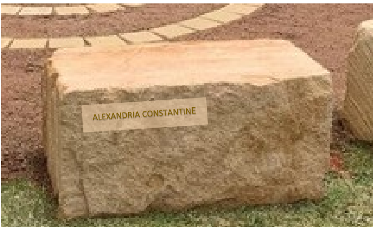
Figure 5: Free standing Grade 1 sandstone block (“log”) 1000 x 500 x 500. the area behind the lettering is to be dressed.
